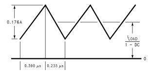
Figure 14. 10 µH Inductor Current, 5V–12V Boost
