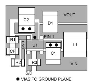
Figure 13. Recommended PCB Component Layout
