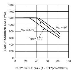
Figure 15. Switch Current Limit vs Duty Cycle
