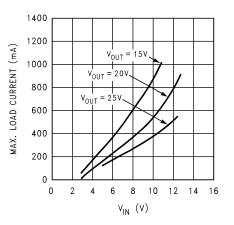
Figure 16. Max. Load Current vs V<sub>IN</sub>
