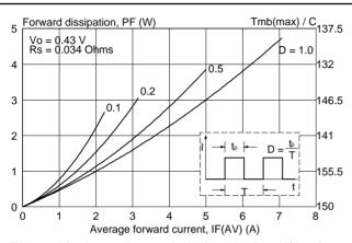
Maximum forward dissipation  $P_F = f(I_{F(AV)})$  per diode; square current waveform where  $I_{F(AV)} = I_{F(RMS)} \times \sqrt{D}$ .
