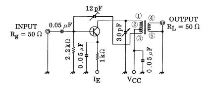
Figure 1 Gpe Test Circuit
