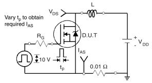
Fig. 14 - Unclamped Inductive Test Circuit
