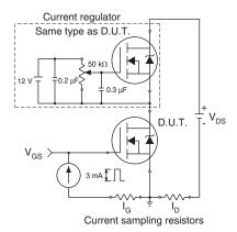
Fig. 17 - Gate Charge Test Circuit
