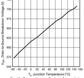
Fig. 10 - Temperature vs. Drain-to-Source Voltage
