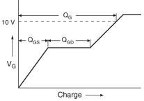
Fig. 16 - Basic Gate Charge Waveform
