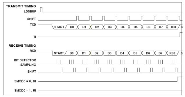
Figure 13-3. Serial Port Mode 2 and 3 Timing Diagram
