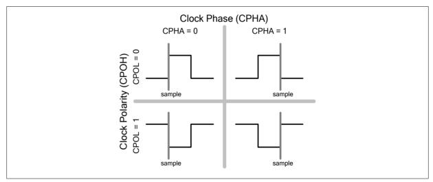
Figure 14-4. SPI Clock Formats
