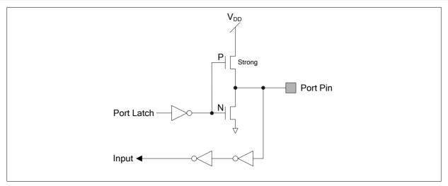
Figure 7-2. Push-Pull Mode Structure
