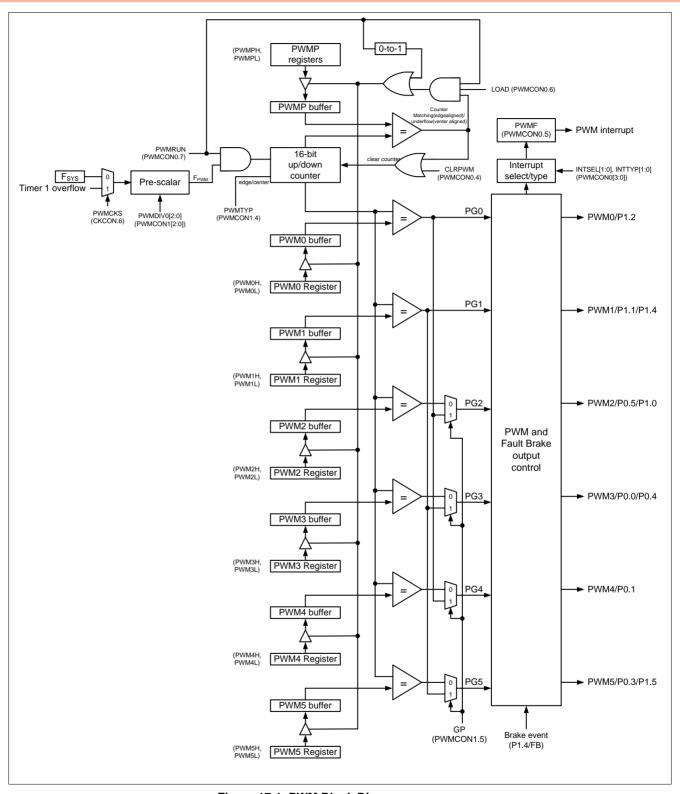
Figure 17-1. PWM Block Diagram
