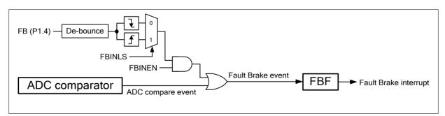
Figure 17-6. Fault Brake Function Block Diagram
