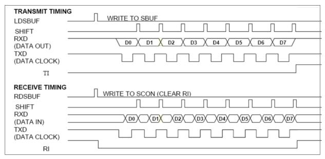
Figure 13-1. Serial Port Mode 0 Timing Diagram
