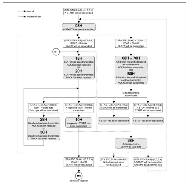
Figure 15-7. Flow and Status of Master Transmitter Mode
