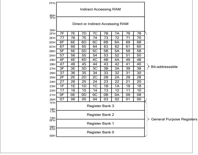
Figure 5-3. Internal 256 Bytes RAM Addressing
