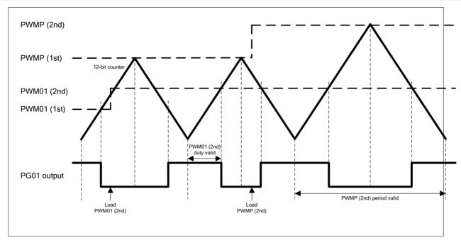
Figure 17-4. PWM Center-aligned Type Waveform
