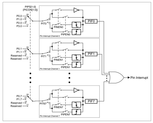
Figure 16-1. Pin Interface Block Diagram
