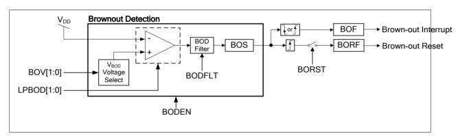
Figure 24-1. Brown-out Detection Block Diagram
