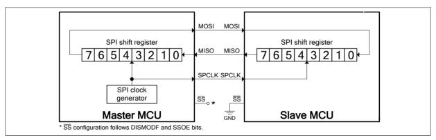
Figure 14-3. SPI Single-Master, Single-Slave Interconnection
