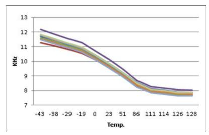
Figure 31-3 LIRC deviation under  $V_{DD} = 2.4 \text{ V}$
