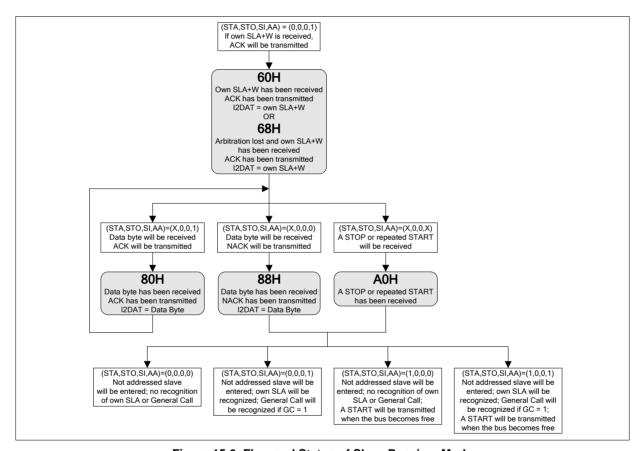
Figure 15-9. Flow and Status of Slave Receiver Mode
