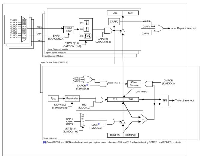
Figure 9-1. Timer 2 Block Diagram
