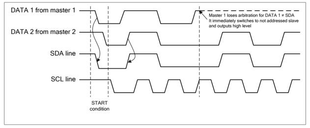
Figure 15-6. Arbitration Procedure of Two Masters
