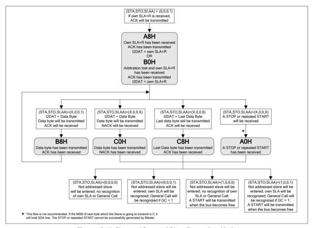
Figure 15-10. Flow and Status of Slave Transmitter Mode
