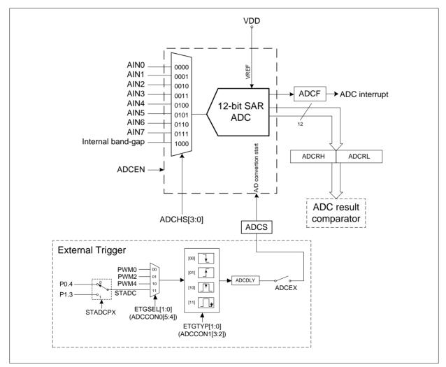
Figure 18-1. 12-bit ADC Block Diagram
