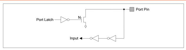
Figure 7-4. Open-Drain Mode Structure
