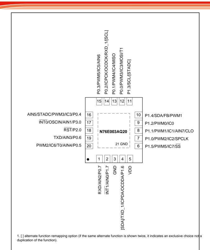
Figure 4-2. Pin Assignment of QFN-20 Package
