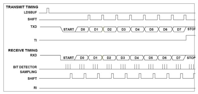
Figure 13-2. Serial Port Mode 1 Timing Diagram
