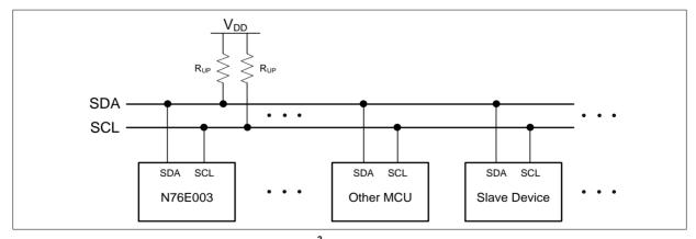
Figure 15-1. I<sup>2</sup>C Bus Interconnection
