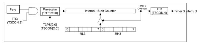
Figure 10-1. Timer 3 Block Diagram
