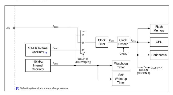
Figure 23-1 Clock System Block Diagram
