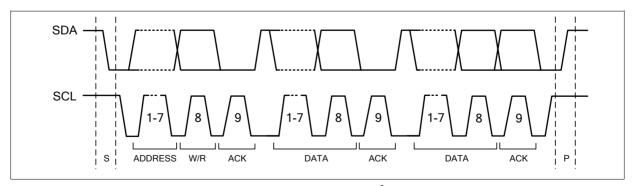
Figure 15-4. Data Format of One I<sup>2</sup>C Transfer
