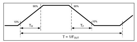
Figure 31-1. I/O A.C. Characteristics Definition
