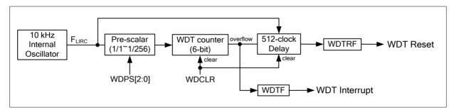
Figure 11-1. WDT as A Time-Out Reset Timer
