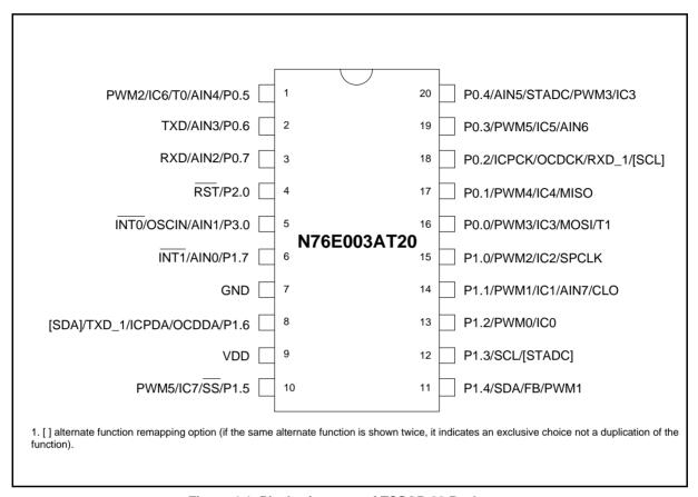
Figure 4-1. Pin Assignment of TSSOP-20 Package
