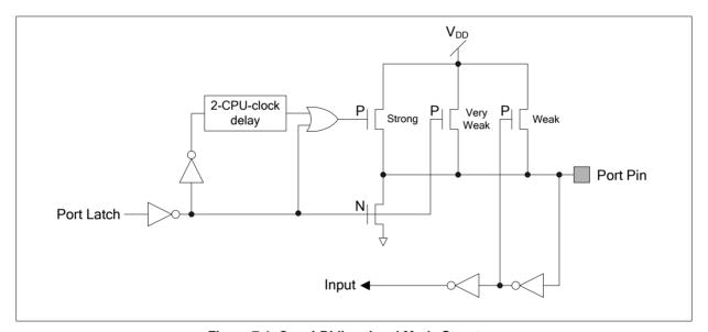
Figure 7-1. Quasi-Bidirectional Mode Structure
