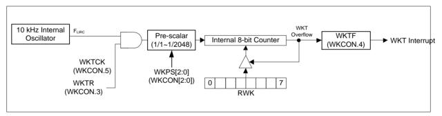
Figure 12-1. Self Wake Up Timer Block Diagram
