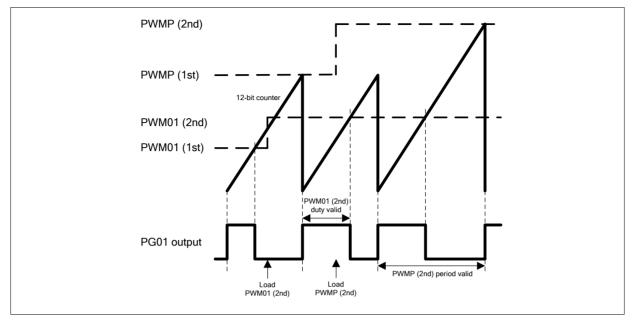
Figure 17-3. PWM Edge-aligned Type Waveform
