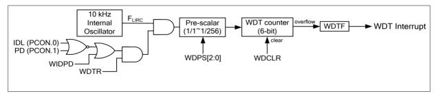
Figure 11-2. Watchdog Timer Block Diagram
