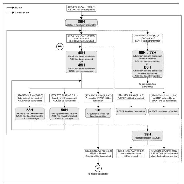
Figure 15-8. Flow and Status of Master Receiver Mode
