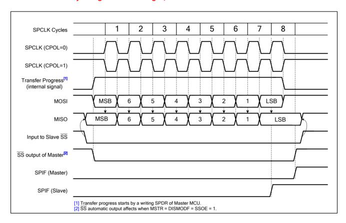
Figure 14-5. SPI Clock and Data Format with CPHA = 0
