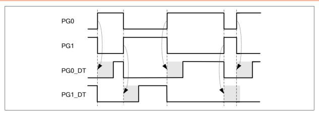
Figure 17-5. PWM Complementary Mode with Dead-time Insertion
