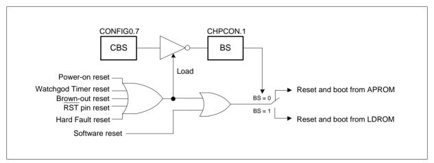
Figure 25-1. Boot Selecting Diagram
