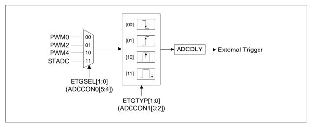
Figure 18-2. External Triggering ADC Circuit
