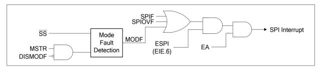
Figure 14-8. SPI Interrupt Request
