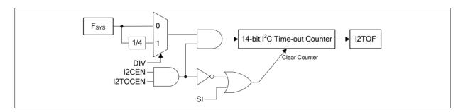
Figure 15-12. I<sup>2</sup>C Time-Out Counter
