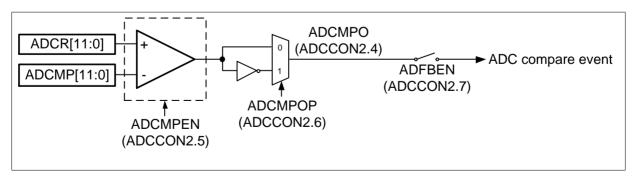
Figure 18-3. ADC Result Comparator
