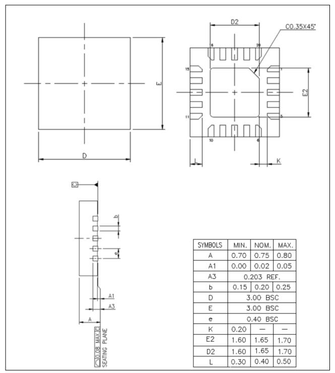
Figure 32-2. QFN-20 Package Dimension
