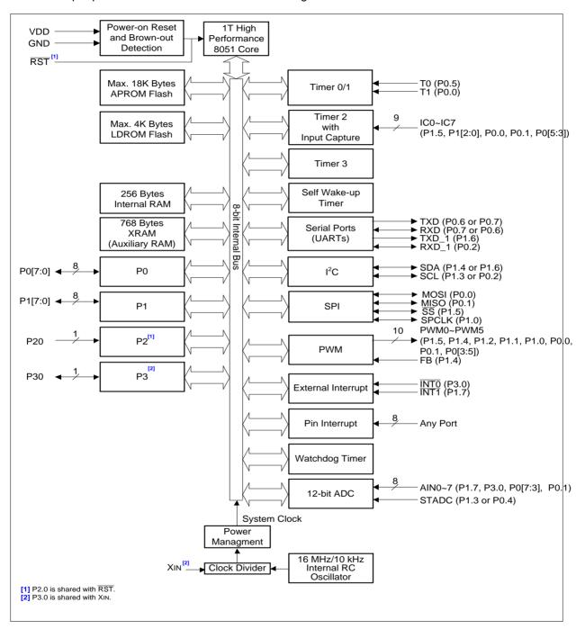
Figure 3-1. Functional Block Diagram
