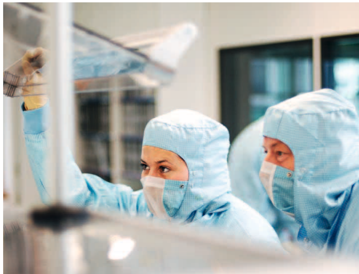
Platinum temperature sensors are produced under clean-room conditions.
