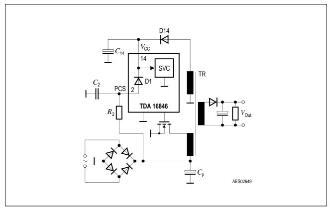
Figure 4 Startup Circuit
