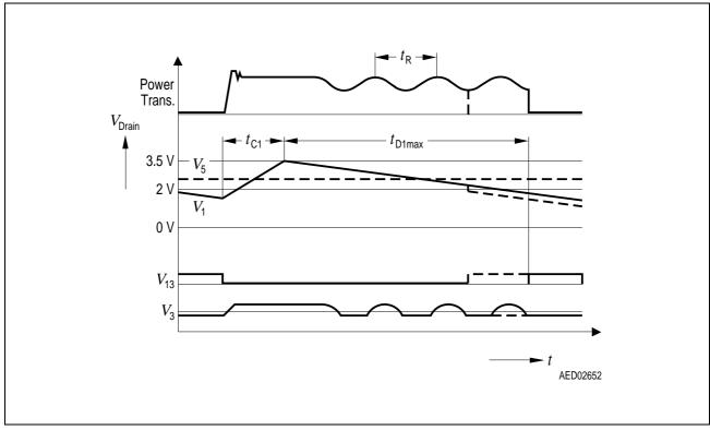
Figure 7 Pulse Diagram of Off-Time-Circuit
