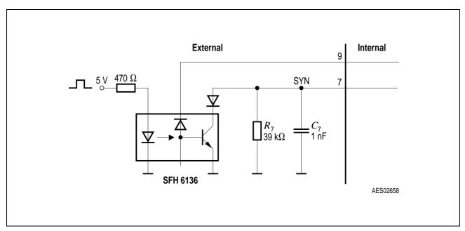
Figure 13 Ext. Synchronization Circuit
