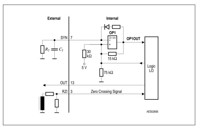
Figure 11 Synchronization and Fixed Frequency Circuit
