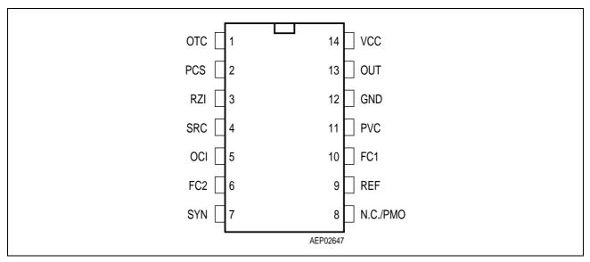
Figure 1 Pin Configuration (top view)
