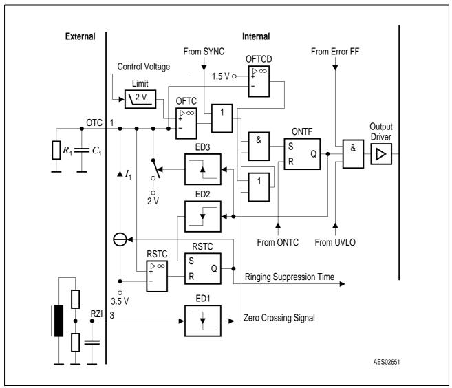
Figure 6 Off-Time-Circuit
