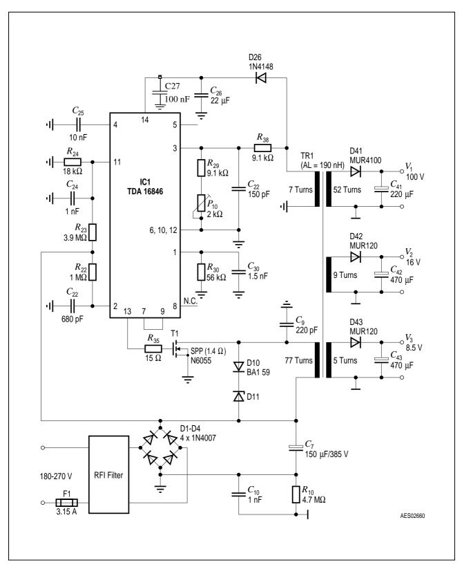
Figure 16 Circuit Diagram for Standard Application
