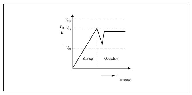
Figure 5 Startup Voltage Diagram
