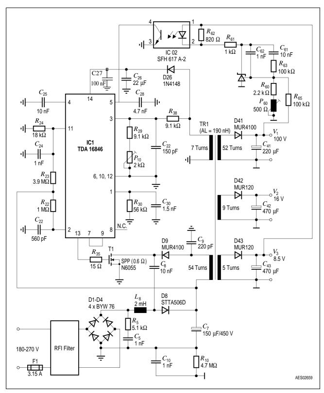
Figure 15 Circuit Diagram for Application with PFC
