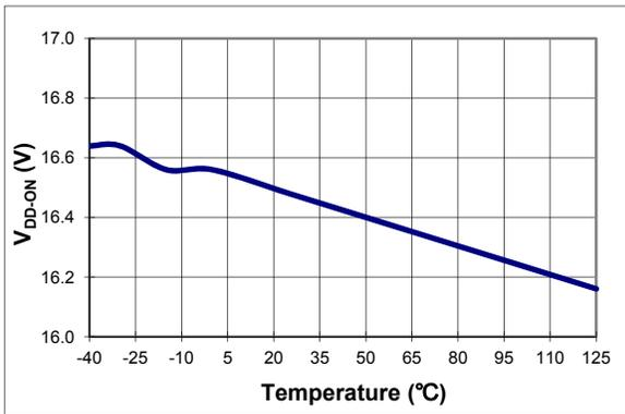
Figure 6. Turn-On Threshold Voltage (V<sub>DD-ON</sub>) vs. Temperature
