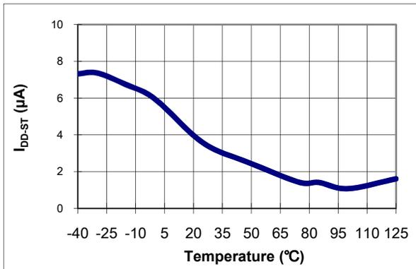
Figure 8. Startup Current (I<sub>DD-ST</sub>) vs. Temperature
