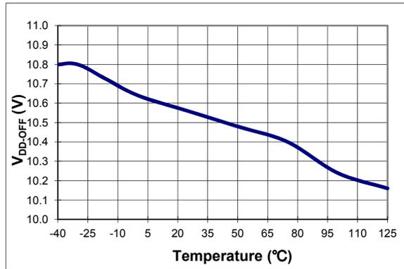
Figure 7. Turn-Off Threshold Voltage (V<sub>DD-OFF</sub>) vs. Temperature
