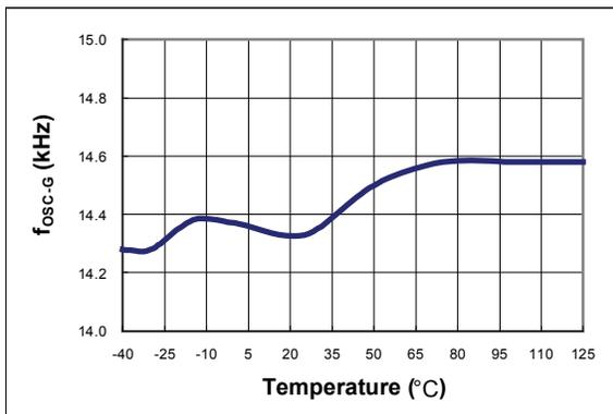
Figure 10. Green-Mode Frequency (f<sub>OSC-G</sub>) vs. Temperature
