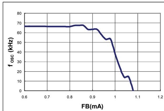
Figure 11. PWM Oscillator Frequency (f<sub>OSC</sub>) vs. FB
