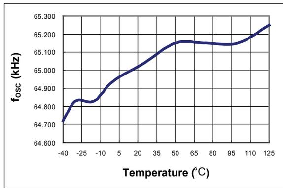
Figure 9. Center Frequency (f<sub>OSC</sub>) vs. Temperature
