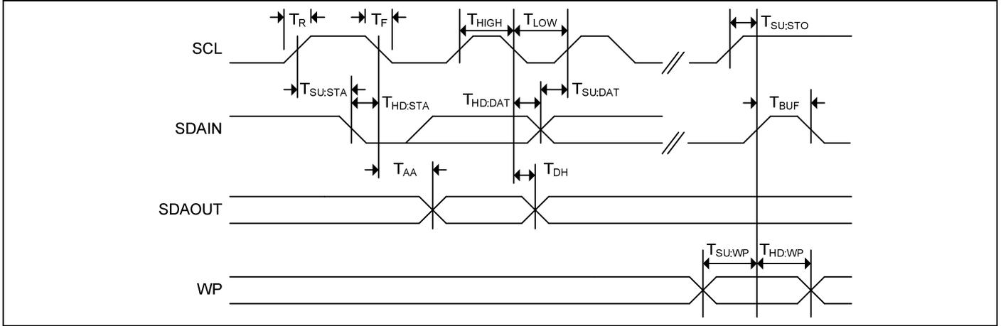
**Figure 1-12. Write Cycle Timing**
