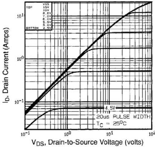
Fig. 1 - Typical Output Characteristics,  $T_C = 25\text{ }^\circ\text{C}$
