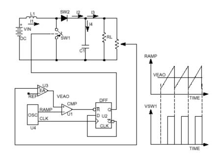
Figure 5. Typical Leading Edge Control Scheme
