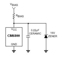
Figure 3. External Component Connections to V<sub>CC</sub>
