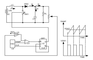
Figure 4. Typical Trailing Edge Control Scheme
