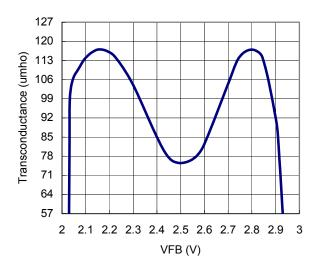
Voltage Error Amplifier  $(g_{mv})$  Transconductance
