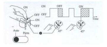
(3) Manual Control ON/OFF(Override Control) Turn the control axis①in direction of arrow by one notechil;QN= OFF=(♥). The manual control is automatically annuled by the counteractifellowin&mmand of the automatic program sequence.
