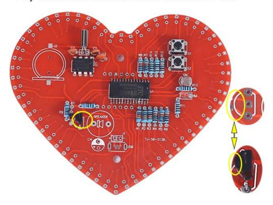
Step 16: Install 1pcs 220uF Electrolytic Capacitor at C4. Pay attention to distinguish between positive and negative. The shorter pin is negative pole and insert into white pad.
