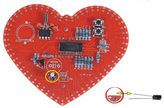
Step 17: Install 1pcs Passive buzzer at SPEAKER. Pay attention to the installation direction.
