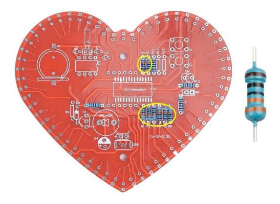
Step 3: Install 1pcs 200Kohm Metal Film Resistor at R13.
