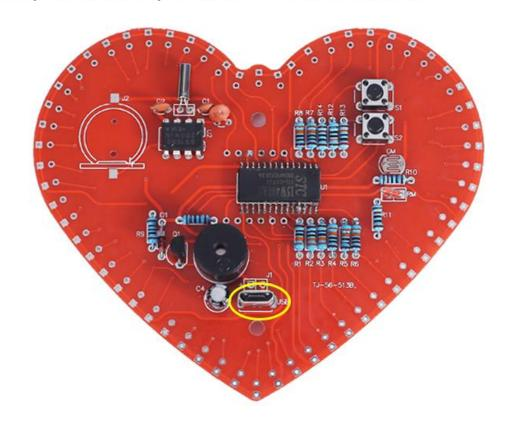
Step 19: Install 1pcs CR1220 Battery Socket at J2.
