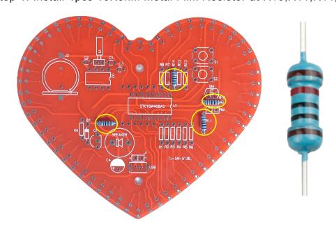
Step 2: Install 8pcs 330ohm Metal Film Resistor at R1-R8.
