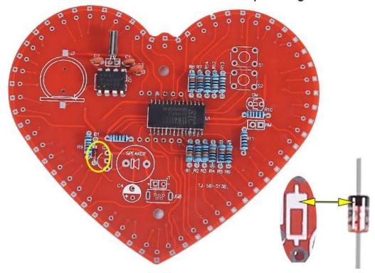
Step 12: Install 1pcs 5516 Photoresistor at GM.
