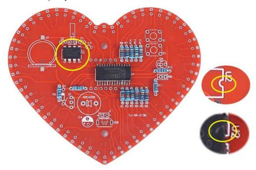
Step 8: Install 1pcs 32.768K Crystal Oscillator at Y1.
