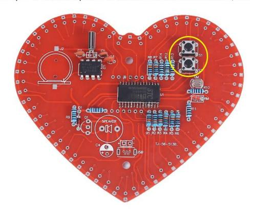
Step 15: Install 1pcs S8550 Transistor at Q1. Pay attention to the installation direction of arc.
