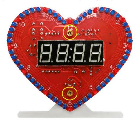
Step 26: Connect the PCB and front acrylic board by 2pcs shorter M3 Screw.
