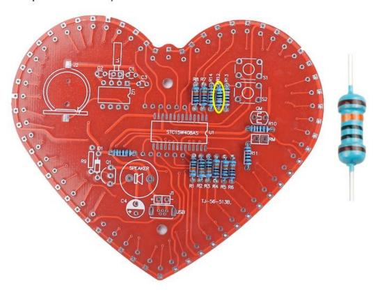
Step 5: Install 1pcs 100ohm Metal Film Resistor at R9.
