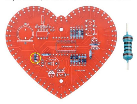
Step 6: Install 1pcs SOP-28 Chip STC15W408AS at U1. There is a mark (circle silk screen printing) on one end of the Chip and there is a mark (curved silk screen printing) on PCB where the Chip can place on. These two marks are corresponding to each other and are used to specify the installation direction
