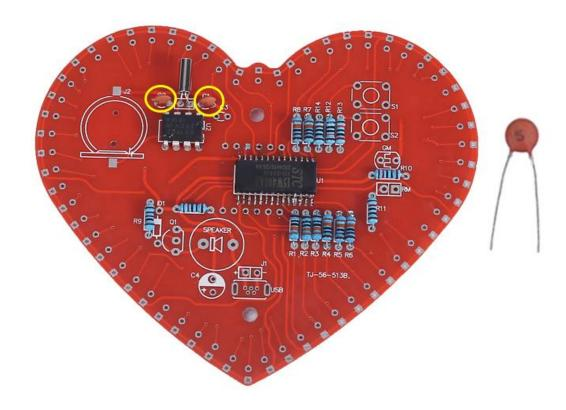
Step 10: Install 1pcs 0.1uF 104 Ceramic Capacitor at C3.
