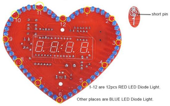
Step 21: Install 1pcs 0.56in 4Bit Digital Tube at SMG on PCB another side. Pay attention to the installation direction of the decimal point.
