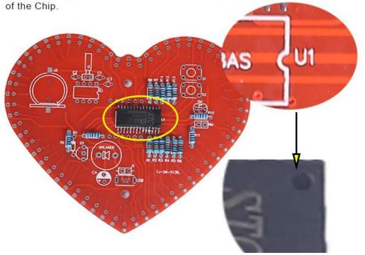
Step 7: Install 1pcs DS1302 Chip at U2. There is a mark (notch) on one end of the chip and there is a mark (curved silk screen printing) on PCB where the IC can place on. These two marks are corresponding to each other and are used to specify the installation direction of the IC.
