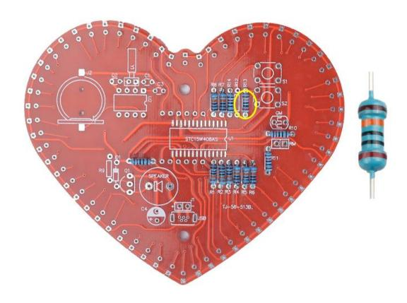
Step 4: Install 1pcs 100Kohm Metal Film Resistor at R12.
