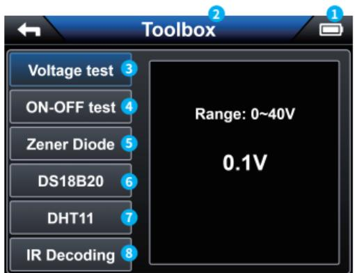
①**Battery display:** This area displays the remaining battery.
