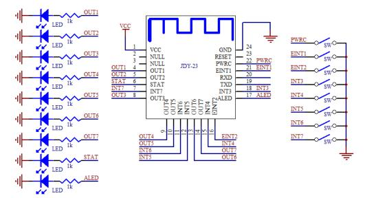
APP can control the high and low level of output pins from OUT1 to OUT7, and APP can read the level state of all input pins of EINT and INT, and EINT1 and EINT2 can actively report the level state in the module connection state.
