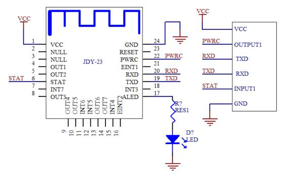
If low power consumption is not required for transparent transmission or disconnection command is not required in connection state, PWRC pin can be disconnected.
