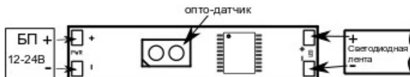
M314.2 are installed at the end of the profile. An optical sensor is located on one side of the sensor, and contacts for connecting a power source and an LED strip or ruler are located on the opposite side.
