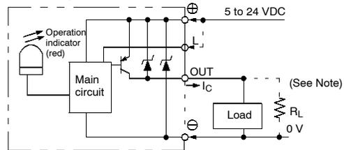
Note: When using a voltage output, always insert a resistor in  $R_L$ .
