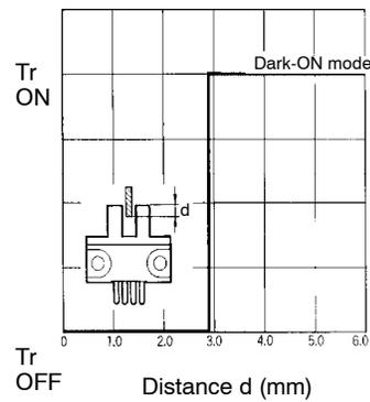
**REPEATED SENSING POSITION CHARACTERISTICS (TYPICAL)**
